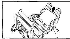
If the film is slack, turn the film cartridge over and tighten it by winding the gears.
